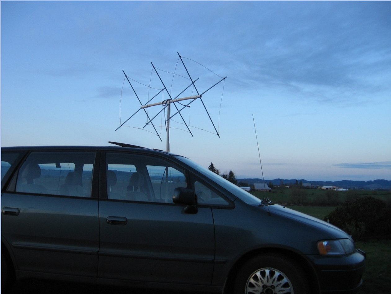
3-Element quad for 121.5 MHz mounted through sunroof.
